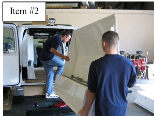
Place Passenger-side Bench/Wall assembly into van so bench rests on wheel well
